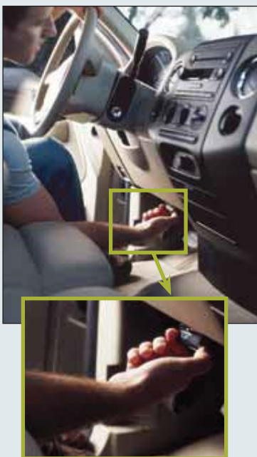
CarChip Pro plugs instantly and unobtrusively into the OBD II port in your car or truck.
