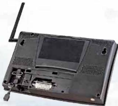
WeatherLink USB data logger installed in Vantage Pro2 Console/Receiver.
