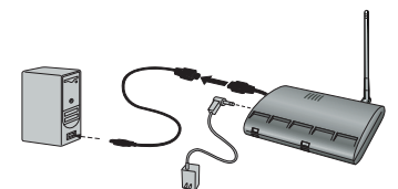
Install Envoy next to your computer using included USB cable and AC adapter.
