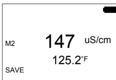
**Note:** The Model pH/EC 80 is equipped with a non-volatile memory that can store up to 50 different sets of readings (pH/Conductivity/TDS/Salinity and temperature). Non-volatile memory will be retained even if power is lost. When all 50 memory locations are used up, the next set of data saved will overwrite the data stored in the first location and so on.
