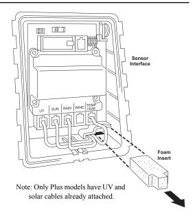
that the foam seals the access port entirely, leaving no holes or gaps large enough for weather or insects. You may have to stack the cables to allow the foam to fit.
