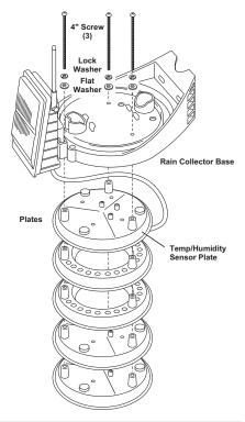
Note: For some models of the ISS, the order in which the five radiation shield plates are assembled may be slightly different than the order shown in the figure. For this reason, ensure that you always reassemble the plates in the same order in which they were disassembled.
