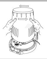
Tip: When new, the cone fits tightly in the base and may require extra pressure to remove. Steady the ISS base between your knees when removing the cone.
