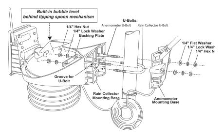
When installing the ISS on a pole, the rain collector /radiation shield section of the ISS and the anemometer can be mounted together as a single unit, or the two sections can be mounted separately.
