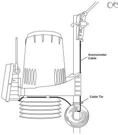
Keep the anemometer cable coiled if possible during the ISS and anemometer assembly so that it is easily stowed once installation is complete.
