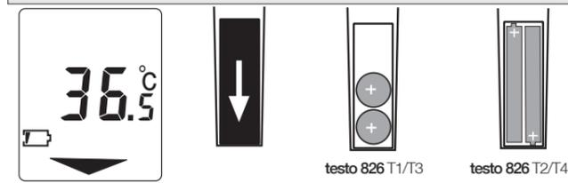
Battery needs to be changed. Observe correct polarisation of batteries/rechargeable batteries.
