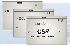
Fuss-free advanced meter options such as Buffer Selection, Switchable Resolutions, Auto-Stable/Auto-Hold Measurment, Unit Selections, etc.
