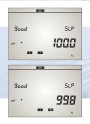
Separate acid and alkaline slope calculation
