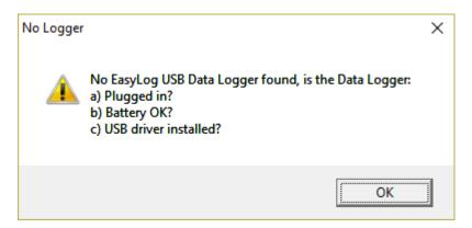
The most likely cause of the above issue is that the battery is flat, particularly if the logger has been in use for over a year and/or is downloaded frequently. Replacing the battery will resolve the issue in most cases.
