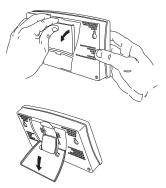
4. Install the two rubber channel feet on the kickstand.
