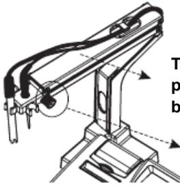
The holder can hold up to 4 probes. The wire of the probe can be fixed to the arm.
