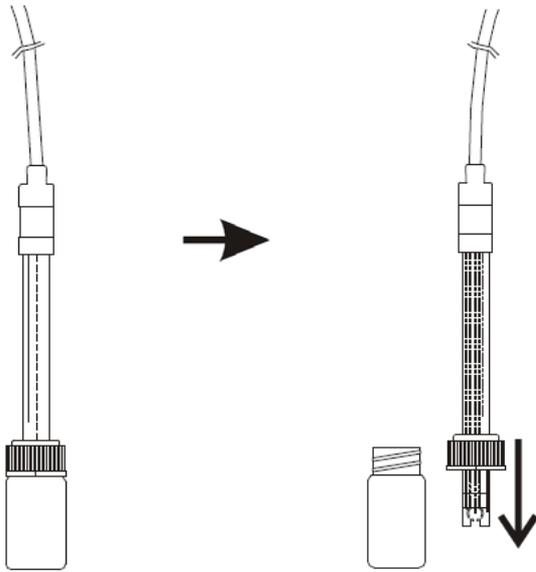
1. Rotate the bottle to remove the bottle from the probe. Pull down the cover and remove it from the probe.
