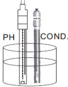
Improper measurement procedure
