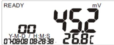
4. Press **MODE** to switch between mV and pH.
