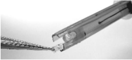
2. Cut the clogged fiber and expose the new portion.
