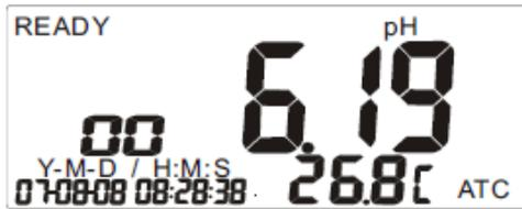
6. Press **MODE** to switch between mV and pH.
