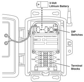
Sensor Interface Module on Soil Moisture Station
