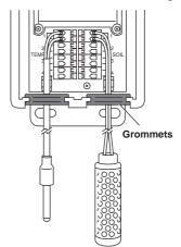
Sensor Cables Run through Grommets
