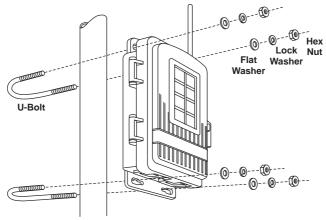
Mounting Soil Moisture Station on a Pole
