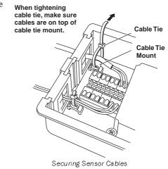
6. To prevent fraying or cutting of cables, secure them so they will not whip about in the wind. Secure a cable to a metal pole by wrapping electrical tape around them both. Make sure cables are secure by placing clips or ties approximately every 3 - 5' (1 - 1.6 m).
