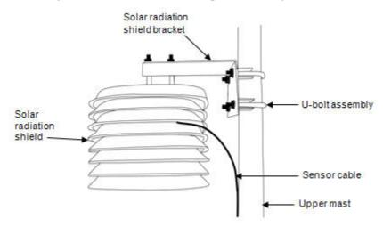
Figure 3: Mounting Solar Radiation Shield
