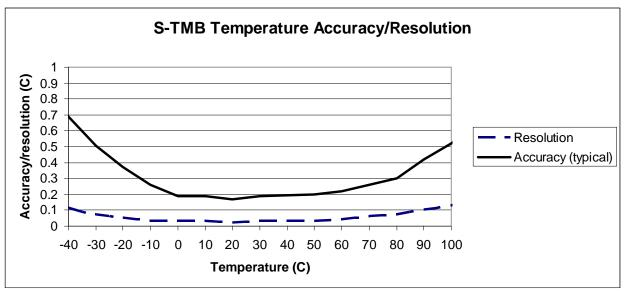
Figure 1: 12-Bit Temperature Smart Sensor Accuracy and Resolution
