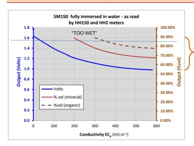
Soil moisture readings are not correct when no soil is present i.e. at 100% vol.
