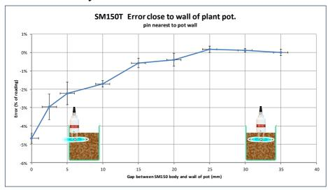
This graph shows the effect of being too close to the wall of a plant pot and gives a partial indication of the shape of the field of sensitivity around the pins
