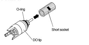
③Attach DO tip to DO electrode body.
