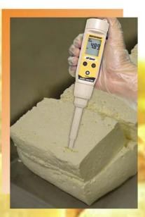
pH is one of the key parameters measured in food processing. The Eutech waterproof pH Spear with tough, spear tip open pore sensor is a rugged, user-friendly tester ideal for direct measurement of solid or semi-solid samples such as cheese, meats, fruits, bread and other similar samples.
