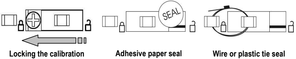
Figure 4-1. Locking and Sealing the Calibration Lock Switch.
