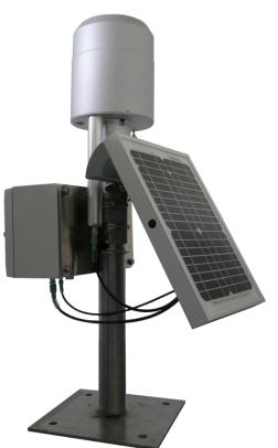
PreLOG – solar powered GPRS precipitation station
