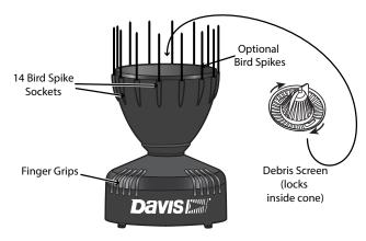
To use the bird spikes, insert one spike into each socket around the rim of the cone. The sockets are tapered: push firmly or tap lightly with a hammer for a secure fit.
