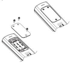
Replace the three 1.5V AAA alkaline batteries located in the battery compartment, observing the indicated polarity.
