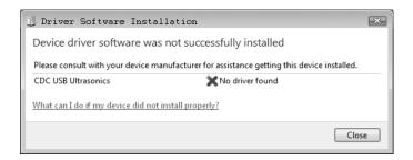
The driver file that needs to be installed can be downloaded directly from our website at <u>www.dakotaultrasonics.comDUsoftware/CDC/CDC\_Ultrasonics.inf</u>, or can be found in the examples folder created on your PC by installing our DakView PC software, and located in the USB directory. The file name is CDC\_Ultrasonics.inf, and can be downloaded and saved anywhere on your local PC.
