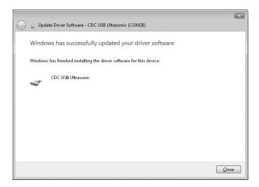
Open device manager again to reference the communications port assigned to the CDC device, it will be displayed to the right of the CDC device. Now that the driver has been successfully installed, a 'keyboard wedge' with serial communications capability can be used to connect to the PZX-7 and will capture the measurements to your PC when the ENTER key is pressed:
