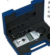
All models are supplied as a complete kit including 6" circumference surface speed wheel, two cone tip adapters, funnel tip adapter, shaft extension, two AA batteries and and an operating instruction manual —all supplied in a foam-fitted carrying case.
