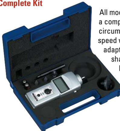
All models are supplied as a complete kit including 6" circumference surface speed wheel, two cone tip adapters, funnel tip adapter, shaft extension, two AA batteries and an operating instruction manual—all supplied in a foam-fitted carrying case.
