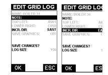
4. Use the UP and DOWN arrow keys to scroll through the Edit options until NOTE or INCR. DIR is highlighted.
