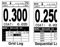
corresponding display view. Notice as the cursor is moved to a different cell, the disr will be updated with the display view saved with the reading. Readings stored in mer ory are indicated by displaying a MEM in the top left corner of the measurement scru
