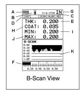
It's important to note that the measurement range on the display be set wide enough, so that the maximum thickness of the material can be viewed on the display. Using the diagram above, if the material thickness was actually 1.75", the underside of the materia would not be viewable according to the current range at  $0.00^{\circ} - 1.00^{\circ}$ . All the user wou see is a black screen from  $0.00^{\circ} - 1.00^{\circ}$  with no view of the bottom contour at 1.75".
