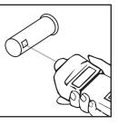
3. Press and hold the Measure Button for several seconds to observe the display as it changes in accordance with the speed of the shaft or rotating element As soon as the laser beam hits the target, the Tachometer will begin displaying speed measurements.
