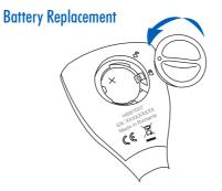
To change the CR2032 lithium battery, turn the battery cover located on the back of the tester counterclockwise to unlock. Remove cover and replace the battery with positive (+) side facina out.
