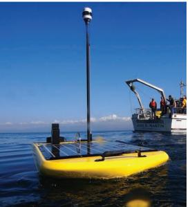
WeatherStation® Multisensor – **Ultrasonic Instrument for Offshore Weather Monitoring**
