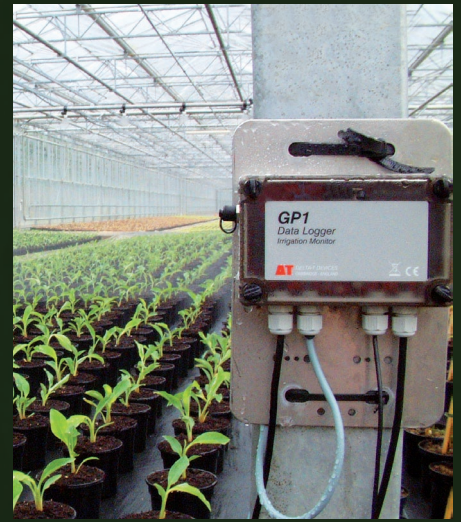
GP1 Data Logger controlling precision gantry irrigation within a glasshouse at Hillier Nurseries.
