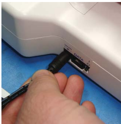
Figure 3-8 Inserting DC power plug.
