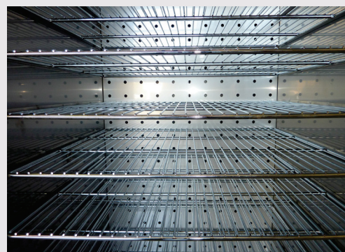
Horizontal air flow system
