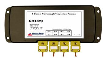
The OctTemp is an eight channel thermocouple data logger with a reading rate of up to 4Hz. It can measure and record 500,000 readings per channel. To maximize memory capacity, users can enable or disable channels. For easy identification, each channel can be named with up to a ten digit title.
