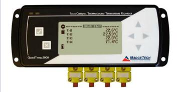
The QuadTemp2000 is a four channel thermocouple data logger with an LCD. The device features onscreen minimum, maximum and average statistics, as well as a user configurable graphics screen that allows for any combination of channels to be displayed. The device accepts J, K, T, E, R, S, B and N type thermocouples.
