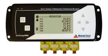
The OctTemp2000 is an eight channel thermocouple data logger with an LCD. The device features onscreen minimum, maximum and average statistics, as well as a user configurable graphics screen that allows for any combination of channels to be displayed. The device accepts J, K, T, E, R, S, B and N type thermocouples.
