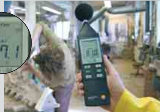
testo 816, Checking noise control
