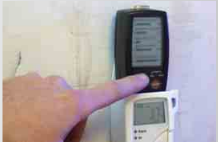
The testo 580 data collects data on site for upload to PC and analysis
