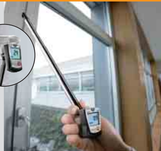
Flow velocity measurement at nontight windows
