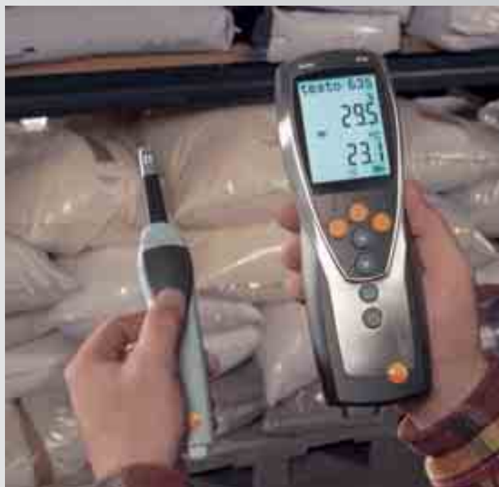
Wireless measurement of warehouse temperature and humidity, with radio handle and attachable humidity probe head
