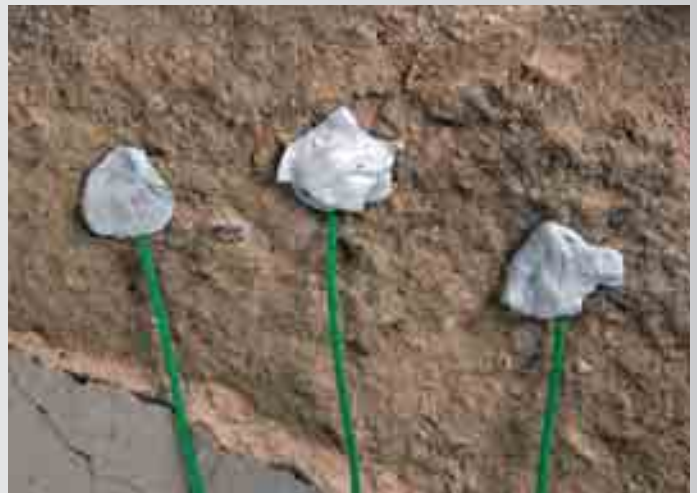
Measures wall surface temperature using three fast-action thermocouple sensors
