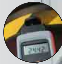
testo 470, mechanical rpm measurement
