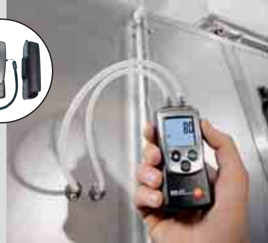
Differential pressure measurement on filters
