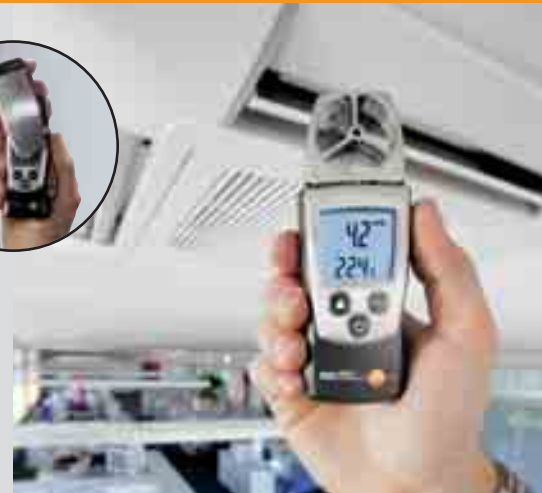
Flow measurement at a duct outlet with 40 mm vane
