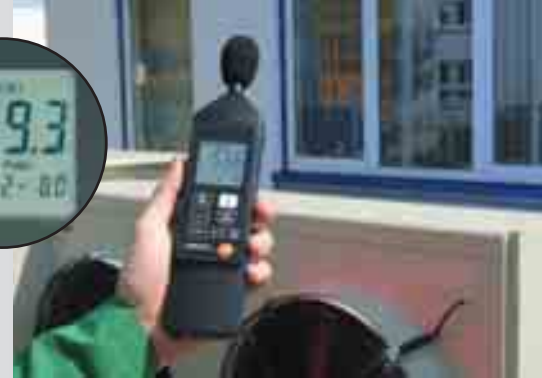
testo 815, Monitoring measurements in ventilation
