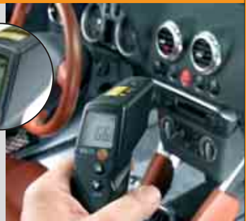
Checking temperature at a ventilator
