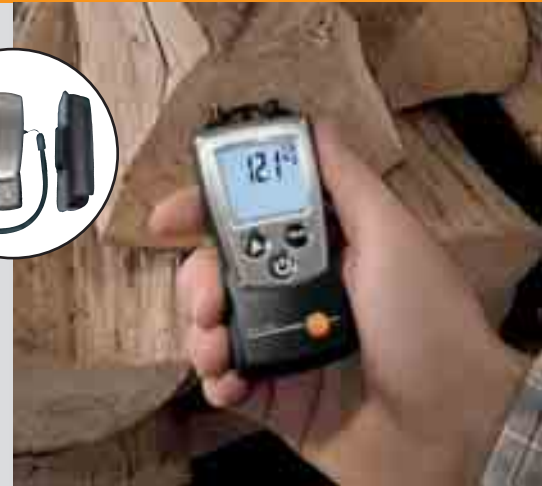
Checking wood moisture
