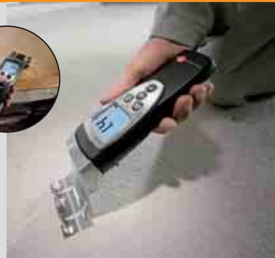
Fast and easy – moisture checks on screed. Measuring several points across a surface ensures more security.
