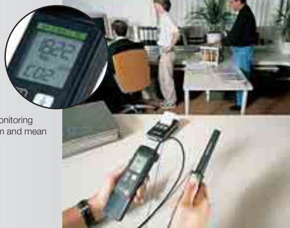
Monitors Indoor Air Quality e.g. in open-plan offices and fast data documentation on Testo printer
