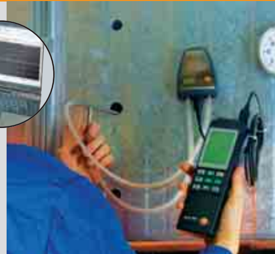
Pitot tube measurement with external 100 Pa probe
