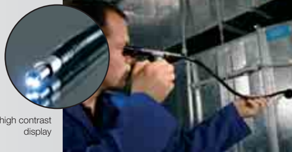
Inspects air duct, with gooseneck casing, middle flexibility
