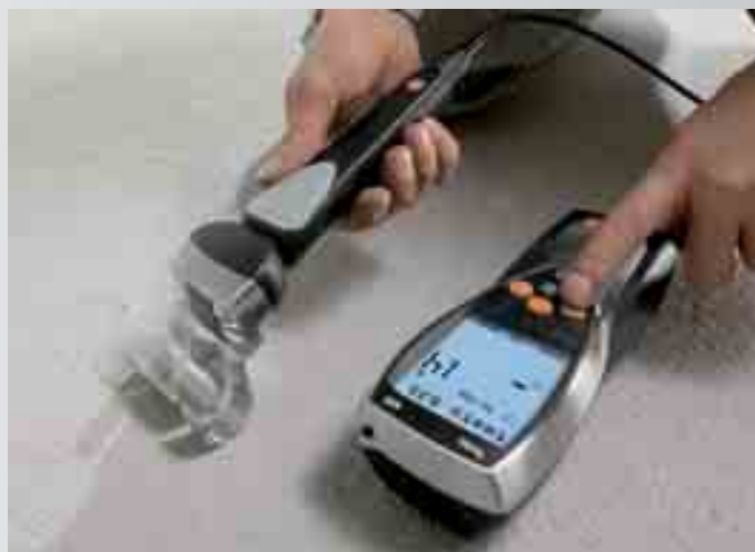
Determining screed moisture quickly and easily. Measuring several points over a surface with the scatter field probe ensures better security of measurement.
