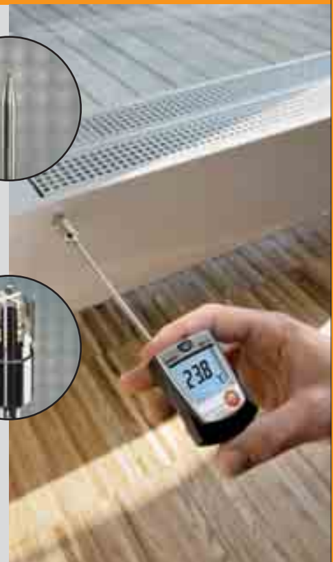
Checking temperature on a radiator
