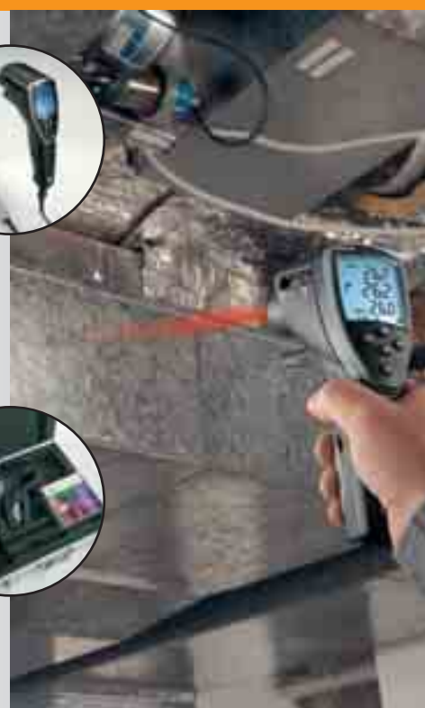
Checks temperature in air conditioning duct
