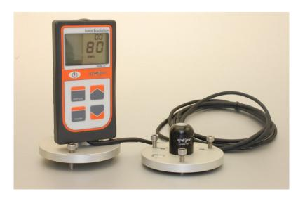
Apogee pyranometers use a silicon cell photodiode and are calibrated to measure total shortwave radiation. The cosine-corrected sensor is designed to maintain its accuracy when radiation comes from low zenith angles.
