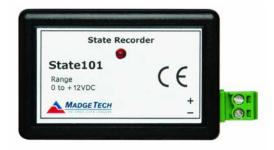
State recorders are useful for collecting data on the duration of an event. The State101 can capture any event that lasts longer than one second. Some typical applications for state recorders include the monitoring of a furnace, air conditioner or pump turning on and off, or even how long a door is left open/closed.
