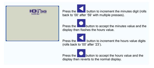
NOTE: It is advised that the real time clock Hours is only adjusted when in STOPPED or READY modes (i.e not recording) to avoid large shifts in day boundary data.
