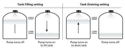
A typical configuration might consist of: High level: 80%, Low level: 20%, High Level Alarm: 90%, Low Level Alarm: 10%, Rapid Level Change Alarm: On (See Alarms section for more information)
