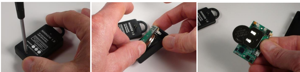
Figure 13: Minnow 1.0 Battery Replacement
