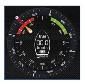
This shows the values of the Real and Apparent wind. The external circle is the compass, showing the north position (in degrees). The internal one is used by the Real and Apparent wind markers (red and yellow respectively) to show the direction from where the wind comes (in d e g r e e s ) .
