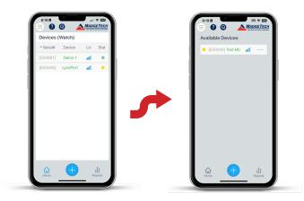
Ensure that Bluetooth is enabled on your smartphone, then press and hold the Bluetooth button on the LynxPro for 3-seconds until the Bluetooth logo appears in the upper left corner. A list of nearby devices will be presented. From this list, locate the LynxPro of interest and tap the desired device to add to your Devices/Home Page.
