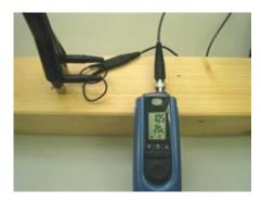
Figure 4-3 Measuring across the fibre direction with M 20
