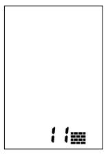
The material index set is displayed together with the symbol for the material moisture.
