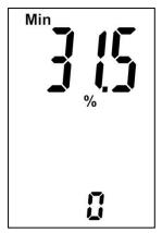
The lowest moisture measurement in a measurement series is displayed together with the "Min" display symbol
