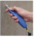
The hand of the operator influences the measurement field of the ball electrode and changes the measured value as it is shown in figure 4-2.
