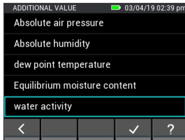
Figure 5-20: Displayable measurements for temperature / humidity sensors
