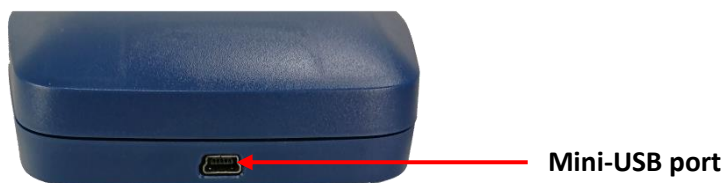
Figure 1-4: Mini-USB port on underside of Hydromette CH 17
