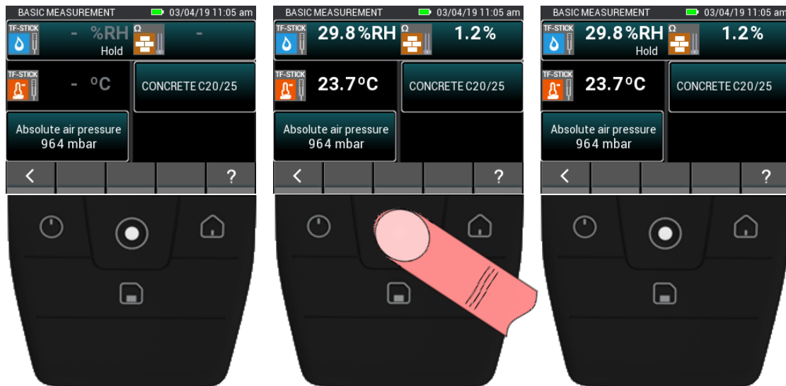
Figure 4-5: Measurement process of the basic measurement
