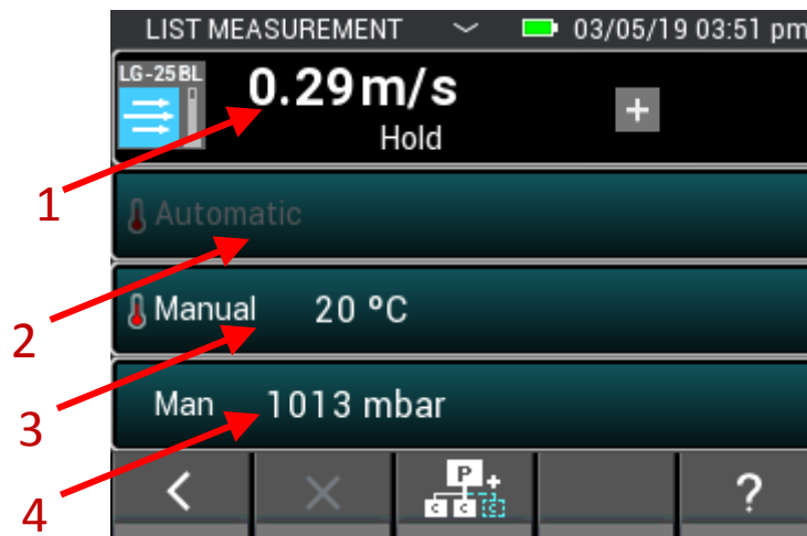
Figure 7-15: Measurement screen of the list measurement with a LG-25 BL air velocity
