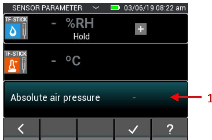
Figure 8-7: Measurement screen of the grid measurement for a TF Stick
