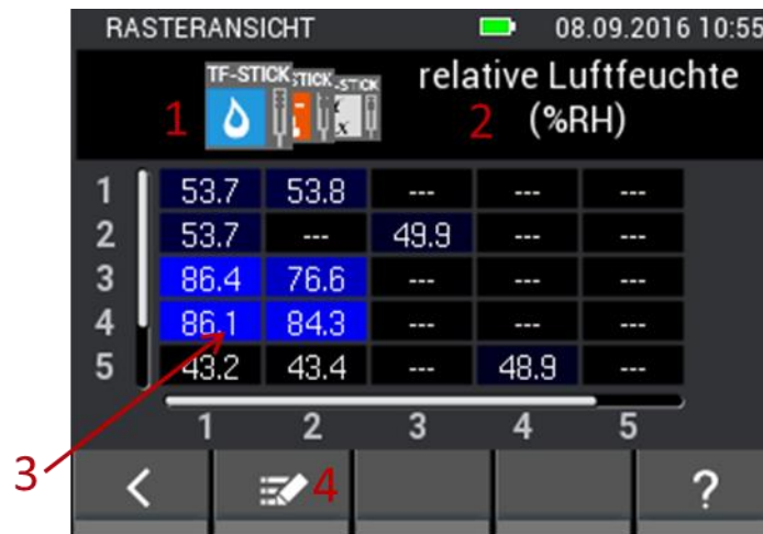
Figure 9-11: Display of the already saved measured values of a grid measurement
