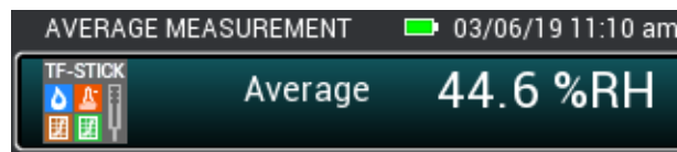
Figure 10-3: Upper button which takes you to the Sensor Selection screen for already selected sensors.
