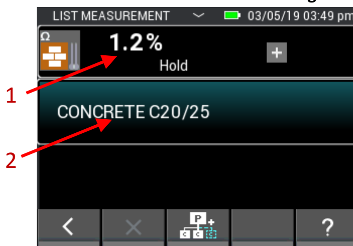
Figure 7-12: Measurement screen of the list measurement with resistance-based moisture content of building materials
