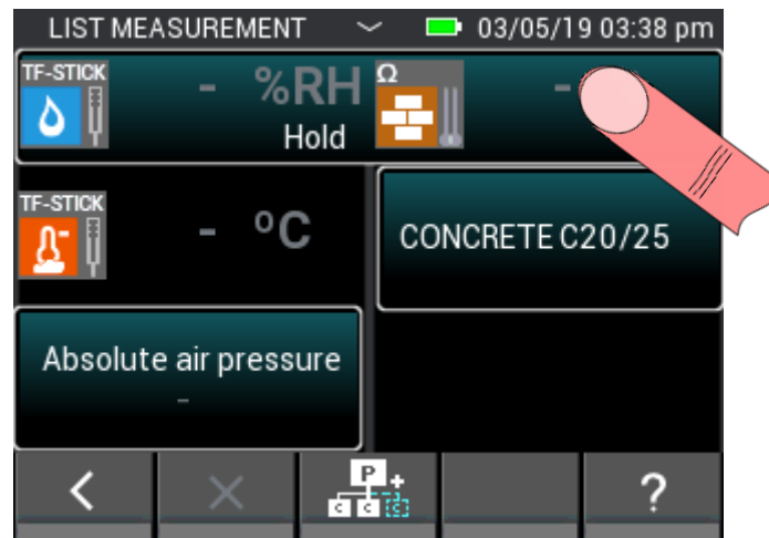
Figure 7-5: Upper button which takes you to the Sensor Selection screen for already selected sensors.
