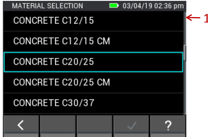
Figure 5-12: Complete building material selection list
