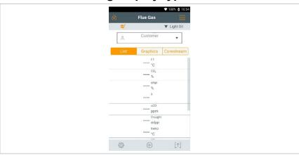
The measurement parameters/units and the number and order of the measurement parameters displayed in the List reading display type can be set, see Section Edit View.
