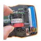
Remove hose connections from the faulty sensor/bridge.
