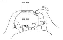
To measure free chlorine in the 0-3.5 mg/L range, remove the disc, mirror and its holder, if pre-installed.
