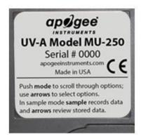
Sensor model number and serial number are located on a label on the backside of the handheld meter.
