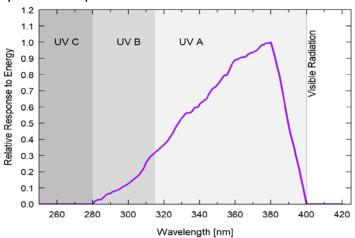
Spectral response estimate of Apogee SU-200 UV-A sensors. Spectral response was modeled from sensitivity of the photodetector and transmittance of the diffuser.
