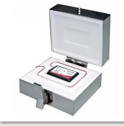
The ThermoVault is a thermally insulated, battery powered, stand alone, thermocouple-based temperature data logger used for the thermal profiling of ovens. The device records temperature data inside an oven to be later downloaded to the user's PC.
