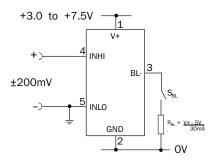
Measuring a single ended input voltage referenced to a split supply, i.e. the input voltage and the meter's power supply share the same OV rail. Ensure solder link LCOM is open.
