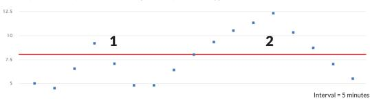
The delay is how many abnormal readings are required to trigger an alarm.
