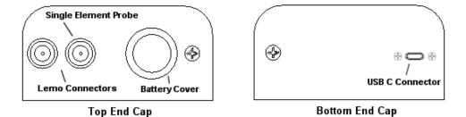
The top end cap is where all connections are made to the **ZX-5 DL**. The diagram above shows the layout and description of the connectors:
