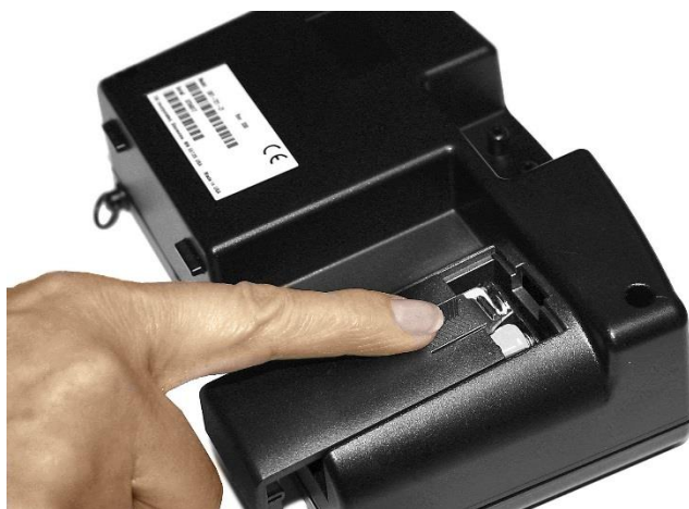
Figure 5: Battery Cover Removal
