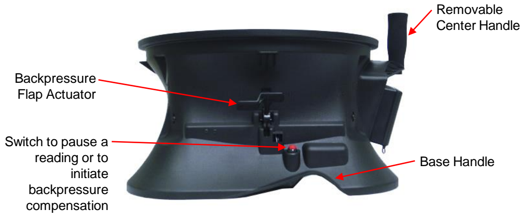
Figure 3: Features of the Model 8380 Base, Side View
